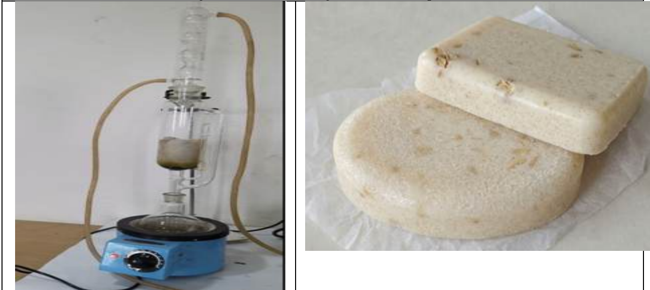
FigureNo.6:Soxhlet Extraction OfC. Borivilianum
